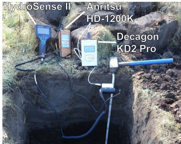
Figure D3. Thermal instruments of Anritsu (thermometer) and a Decagon Devices KD2 Pro installed in a soil pit. Volumetric water content was determined alongside using a Campbell HydroSense I or II (here II).
