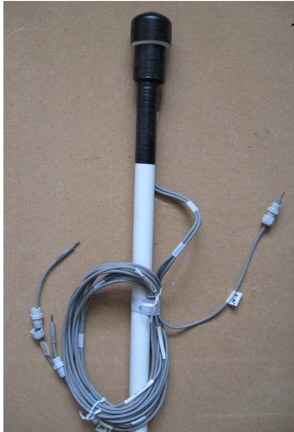
Figure D5. HOBO thermistor chain construction before installation in borehole. Construction consists of four thermistors that wired and held in place at specific and predefined depths within a PVC tube of 50 mm diameter that is filled with dry sand before installation.
