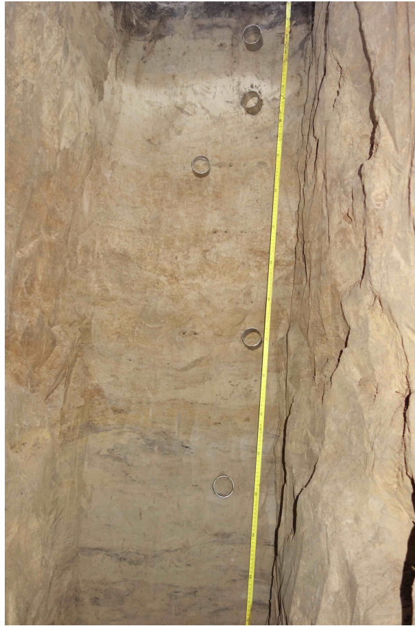
Figure D4. Soil pit "pit-2017-RB-2" with metal cylinders for soil soil sampling. Old radiocarbon ages of topsoil (upper two sampling cylinders) were determined while subsequent samples show older ages with depth.
