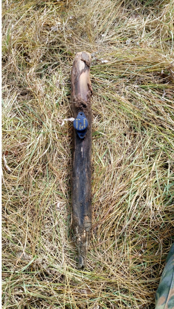
Figure D1. Proges Plus Thermo Buttons 22L (TB) attached on wooden peg. Installation by pushing or hammering into the soil to a depth of approximately 5 cm.
