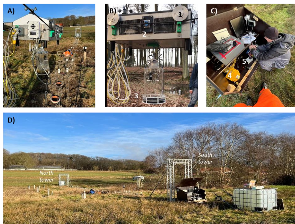
Figure 5: A) The SkyLine2D trolley and chamber at Vejrumbro site looking from south towards the north tower. Note the orange collars on the ground arranged in a straight line. B) Close-up of the chamber: wheels move the trolley back and forth on the ropes (1), magnet sensors (2) and rubber gasket on the bottom of the chamber (3). C) The analyzer “hut” with the Picarro G2508 gas concentration analyzer (4) and the main pump (5). D) The SkyLine2D system with the north and south towers and the analyzer shelter. Towers were at both ends attached with ropes to water-filled 1000 L pallet tanks. One tank shown at the right of the picture.
