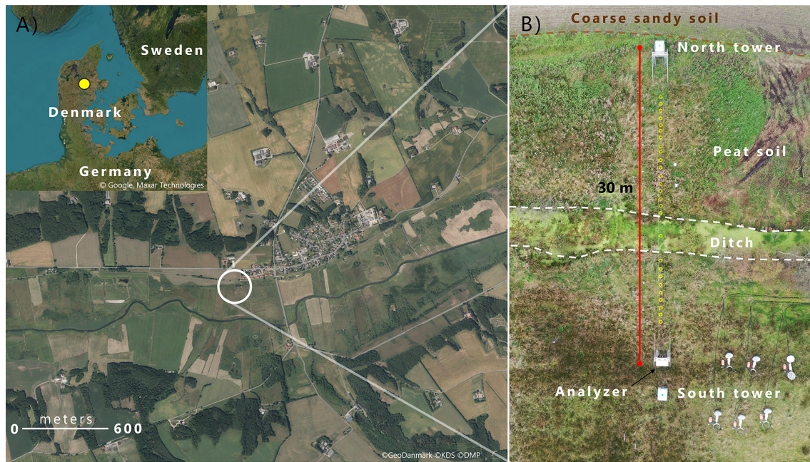
Figure 1. (A) The Vejrumbro location in Jutland (N 56.43819 E 9.54527 (WGS 84)) in the Nørre Å valley near the village of Vejrumbro. The grey circle marks the placement of the SkyLine2D system. Satellite images: © Google Earth. (B) Drone image of the measurement transect (27 September 2023) after flux measurements had stopped. Dashed brown line marks the approximate boundary between the agricultural field, coarse sandy soil (north) and the peat/organic soil (south). The red line marks the end points of the SkyLine2D system (30 m). The open yellow circles ( n = 27 ) mark the approximate position of individual collars across the transect of the field (24 m in length) where greenhouse gas fluxes were measured. The ditch is located between the dashed white lines. The analyzer was placed at the south tower. Elevation above sea level along the 24 m collar transect varied from 3.77 m in the south to 4.06 m in the north.
