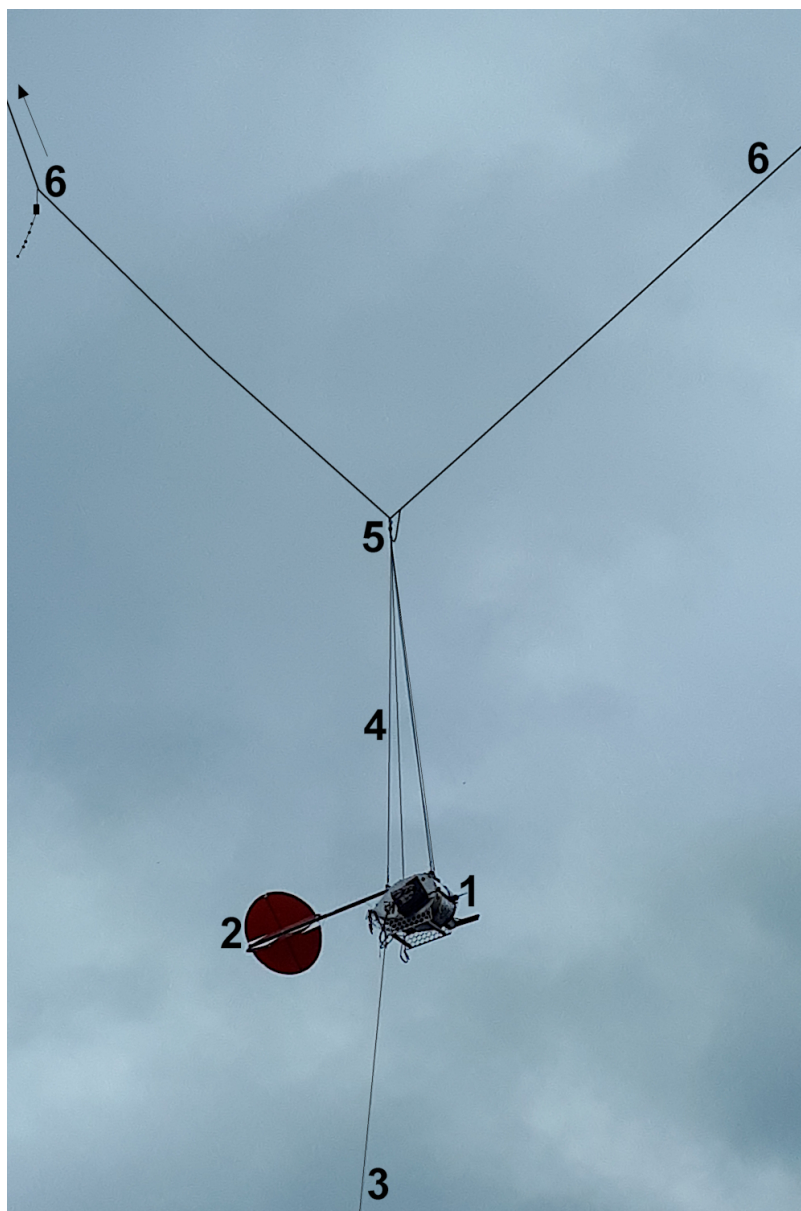
Figure 2. MPCK + instrument (1) with stabiliser fin (2) hanging on four line segments (4) connected to the main tether (6) by a knot (5). It has a handling line (3) hanging below for guiding it during take-off and landing. The arrow next to the main tether (6) points towards the two Helikites.
