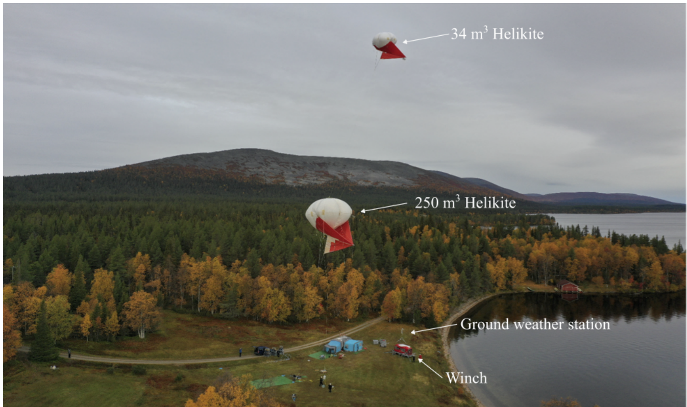
Figure 1. The Max Planck CloudKite (MPCK) platform, and the ground weather station at Pallasjärvi during PaCE 2022.
