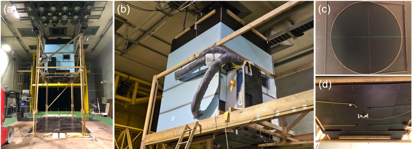
Figure 332. a) IJP mounted on a wooden frame in the testing chamber; b) zoom-in on the IJP and air conditioning unit; c) open nozzle with honeycomb; d) closed nozzle with louvers.
