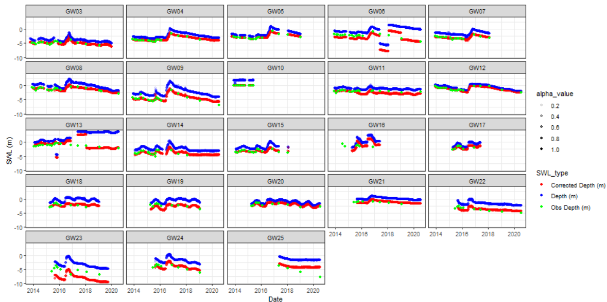
Figure S1: Groundwater level logger data corrected for cable length and automatically matched to observed data.
