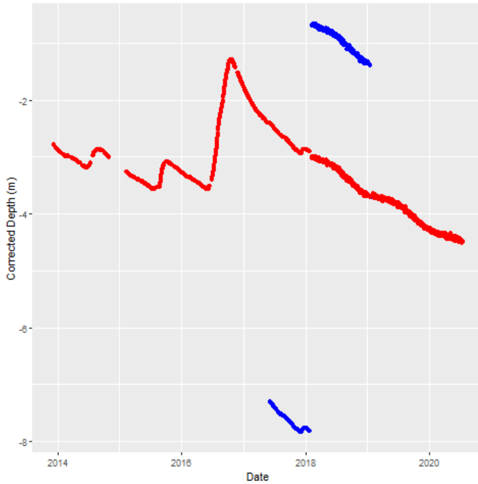
Figure S4: Second correction of the GW06 groundwater level data
