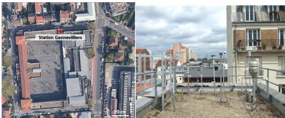
Figure S14: Map specifying the location of the Gennevilliers station (left) and a photograph (credit: AirParif) of the sampling heads on the roof of Louis Pasteur College (right).
