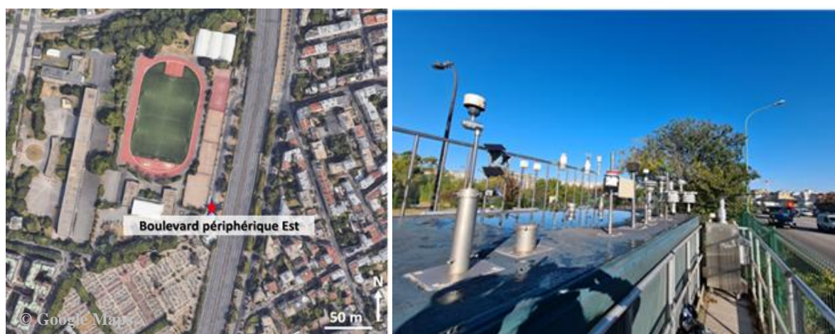
Figure S13: Map detailing the location of the BPEST station (left) and a photograph (credit: AirParif) of the sampling heads at the edge of the ring road (right).
