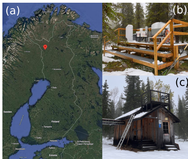
Figure 1. (a) Map of Finland showing the location of the Kenttäröva station (© Google Maps 2024), (b) photograph of the platform with instruments, and (c) photograph of the cabin with a Vaisala CL31 ceilometer on the roof.
