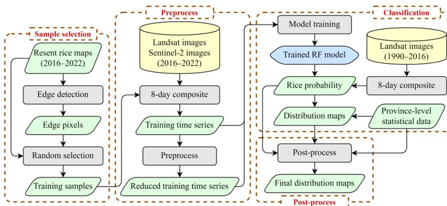
Figure 3: The conceptual flowchart of the method.
