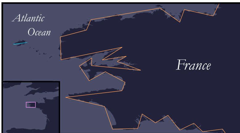
Figure 13. Illustration of the Douglas-Peucker geometric data compression algorithm for coastline simplification at three levels of resolution.
