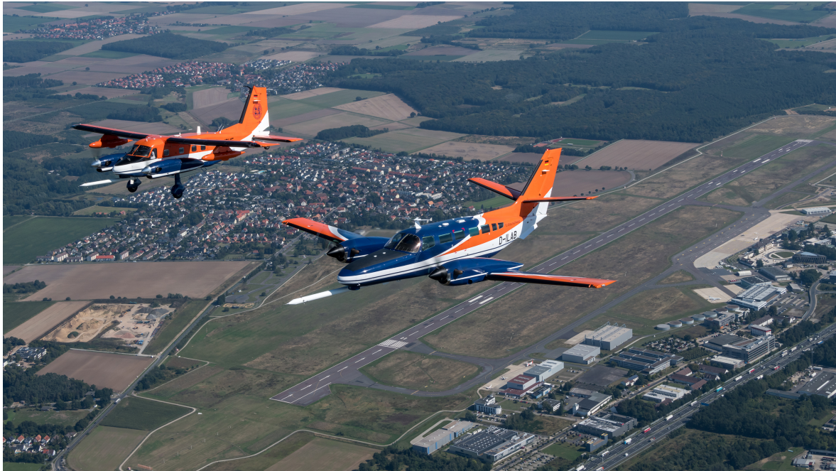
Figure 1. The research aircraft Dornier 128 D-IBUF (left) and Cessna F406 D-ILAB (right) with striking painting for good visibility and the characteristic nose boom for meteorological measurements flying above their home base, the airport Braunschweig. Florian Szczepanek, AviationMedia.com
