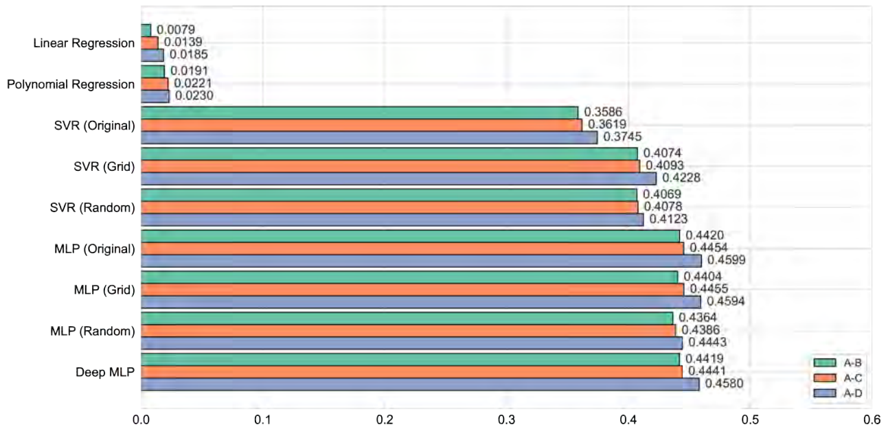
Figure 12. Performance comparisons for regression models applied to GEBCO (A) with curv curv SWOT (B), SIO V32.1 (C), and SDUSTVGGA (D). R^2 values are shown for Linear Regression, Polynomial Regression, SVR, and MLP methods, where the MLP used three hidden layers (200, 200, 100 neurons) and Deep MLP used seven hidden layers (512, 512, 256, 256, 128, 128, 64 neurons).
