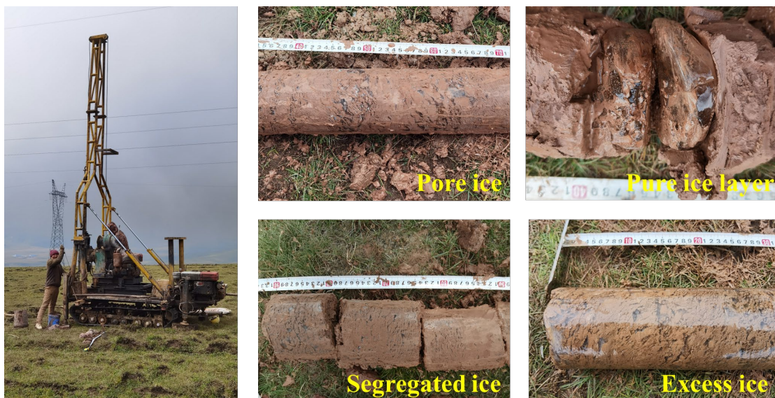
230 Figure 3: Field permafrost drilling work and various types of ground ice obtained during drilling.
