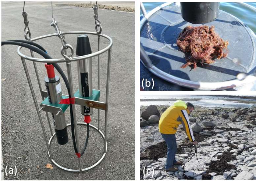
Figure 2: Ramses two sensor measurement set (a), L_u sensor installed to the measuring frame while conducting measurements (b), L_u sensor held in hand while conducting measurements (c).
