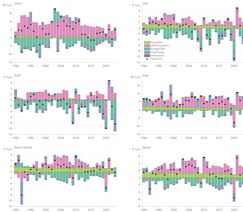
Figure 17. Kaya decomposition of the main drivers of fossil CO 2 emissions, considering population, GDP per person, Energy per GDP, and CO 2 emissions per energy, for China (top left), USA (top right), EU27 (middle left), India (middle right), Rest of the World (bottom left), and World (bottom right). Black dots are the annual fossil CO 2 emissions growth rate, coloured bars are the contributions from the different drivers to this growth rate. A general trend is that population and GDP growth put upward pressure on emissions (positive values), while energy per GDP and, more recently, CO 2 emissions per energy put downward pressure on emissions (negative values). Both the COVID-19 induced drop during 2020 and the recovery in 2021 led to a stark contrast to previous years, with different drivers in each region.
