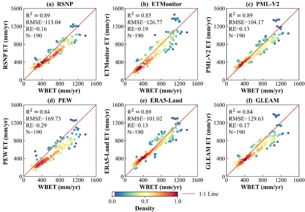
**Figure 6: Comparison of estimated ET and WBET over 38 basins. The relative mean square error (RMSE) and bias are both in mm/yr.**
