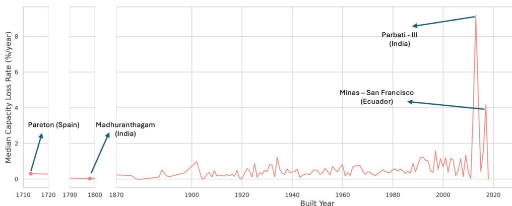
370 Figure 7: Median capacity loss rate for each year of construction among the GRILSS reservoirs. The x-axis shows two distinct kinks corresponding to the two reservoirs built in the 18th century. Reservoir names are indicated for those constructed in that century and for any that exhibit anomalously high capacity loss rates relative to the overall trend.
