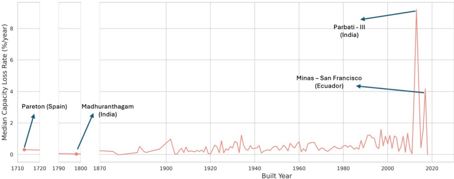
Figure 7: Median capacity loss rate for each year of construction among the GRILSS reservoirs. The x-axis shows two distinct kinks corresponding to the two reservoirs built in the 18th century. Reservoir names are indicated for those constructed in that century and for any that exhibit anomalously high capacity loss rates relative to the overall trend.
