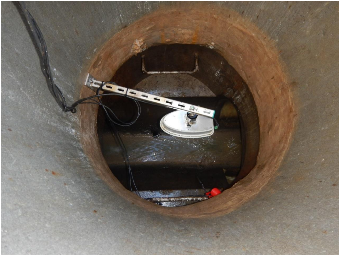
Figure S 26: Sommer SQ-3 flow meter in a “low-flow” measurement site.
