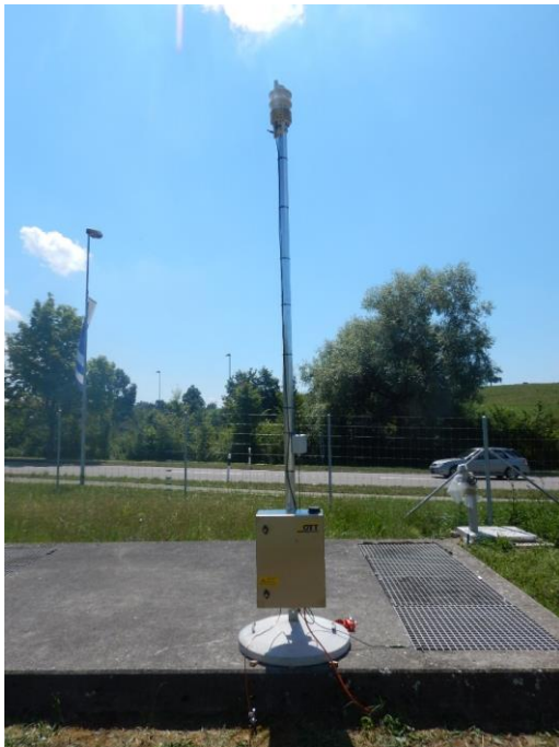
Figure S 32: WS-700 on post with concrete base.
