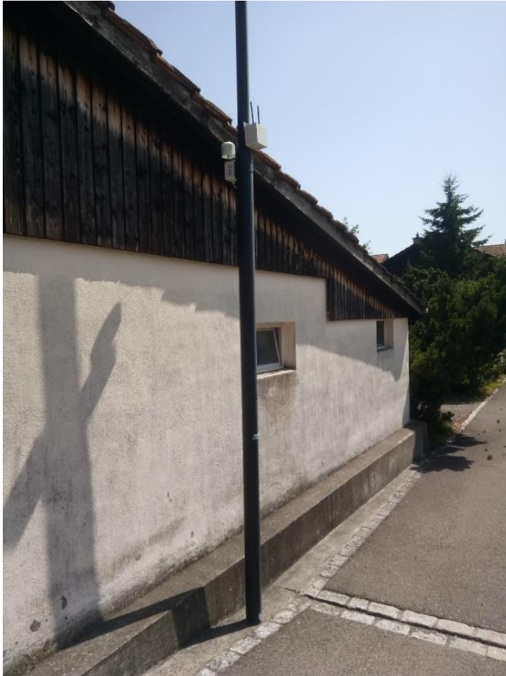
Figure S 28: Ambient temperature and humidity sensor mounted at a lamp pole (backside).
