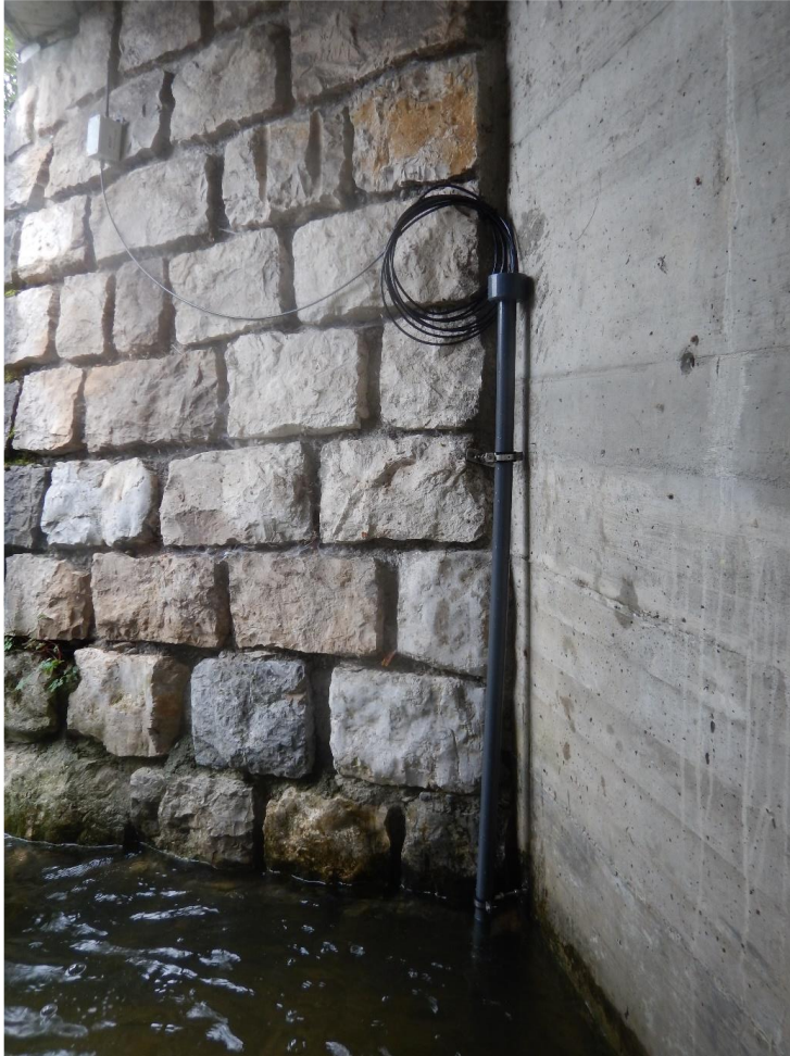
Figure S 29: Pressure probe inside a protective hull connected with the LoRaWAN-logger
