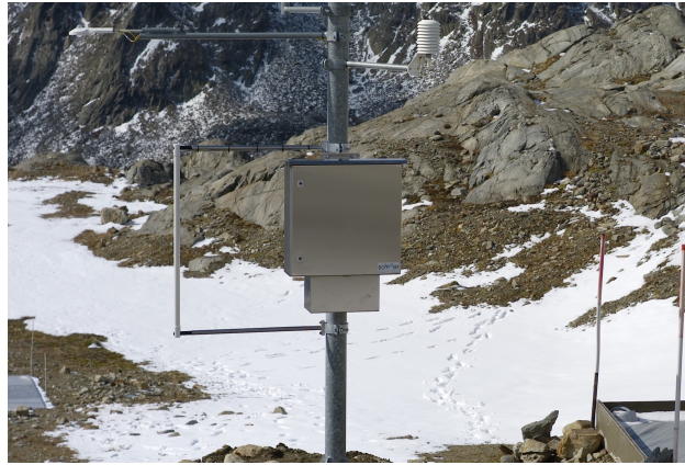
Figure 10. The SND snow drift sensor installation at the Bella Vista AWSS. The sensor elements are placed in the cylindrical tube that is vertically held in place by two mounting arms building a rectangular shape (left of the logger box). In the background (lower left in the photo), the snow scale in the slight depression is visible (sheltered site, sink for snow deposition). The snow pillow besides the main AWSS mast (lower right in the picture) measures SWE at the exposed location.
