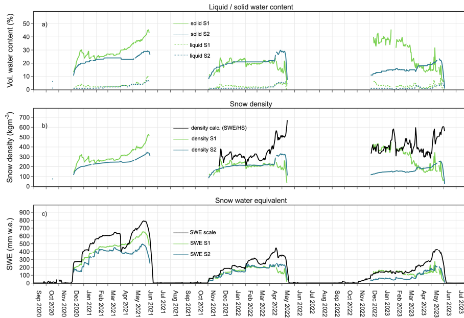
Figure 9. Liquid and solid water content measured by SPA (a), snow density as measured by SPA and calculated from independent measurements of SWE and HS (b), and SWE measured by SPA and by the snow scale (c). All data: hourly averages at the Proviandepot station from Nov 25, 2020 to Dec 31, 2020. S1 is data from the diagonally spanned flat band , S2 from the flat band that is spanned horizontally 10 cm above the ground . S1 data is filtered for HS below 30 cm, S2 for HS below 20 cm. Calculated density in (b) is not available in winter 2020/2021 because HS data from the SPA was not logged before July 2021.
