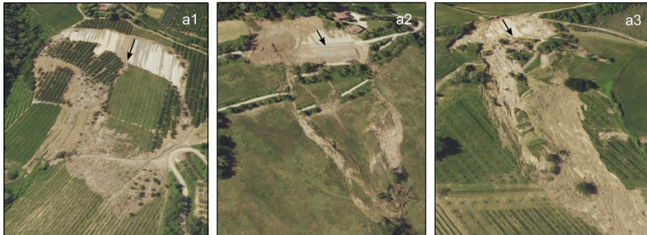
RS1) Fully-developed rock-block slides
