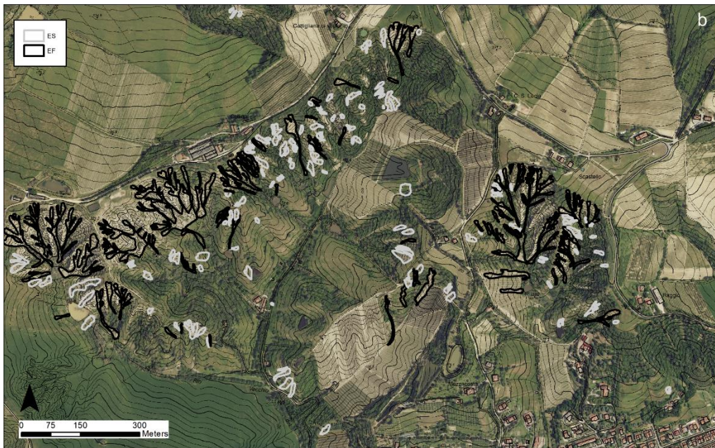
Fig. 15. Example images from the landslide inventory showing two representative area in coarse-grained units (a) and in fine-grained units (b). DS1=debris slide with high mobility; DS2=debris slide with low mobility; DF1=debris flow with high fluidity; DF2=debris flow with low fluidity; RS1=fully-developed rock-block slide; RS2=incipient rock-block slide; ES=earth slide; EF=earth flow.
