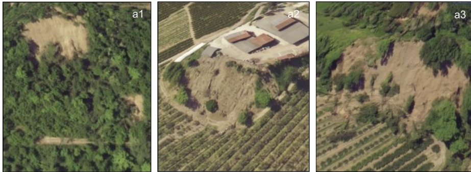
DS1) Debris slides with high-mobility causing complete vegetation removal
