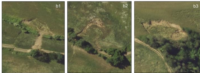
Fig. 5. Representative images of the two distinct types of debris slides caused by the May 2023 event.
