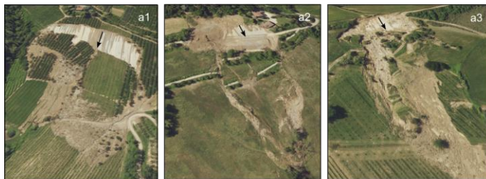
RS2) Incipient rock-block slides
