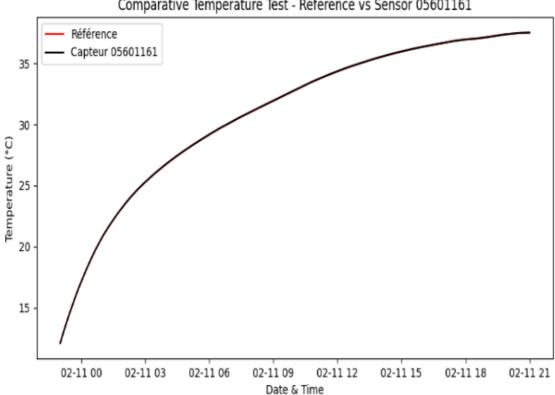
Comparative Temperature Test - Reference vs Sensor 05601161
