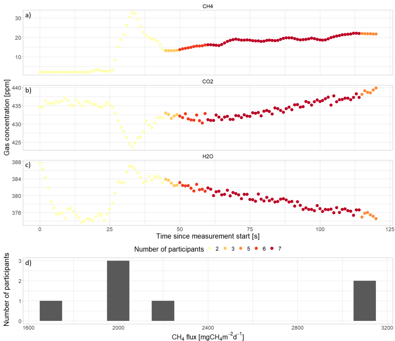
Figure B6: Measurement example VQC8 of an overall increase in CH 4 concentrations over the time of the chamber closure after a strong jump in CH 4 concentrations. Simultaneous measurements of CH 4 (a), CO 2 (b), and H 2 O (c) concentrations over time during chamber closure with the colors of the data points indicating how many participants included the respective data point in the time period that they chose for flux calculation. Only the responses by participants who gave start and end times for flux calculation were considered for this figure. Histogram of CH 4 fluxes calculated based on the time period chosen for flux calculation by the participants (d).
