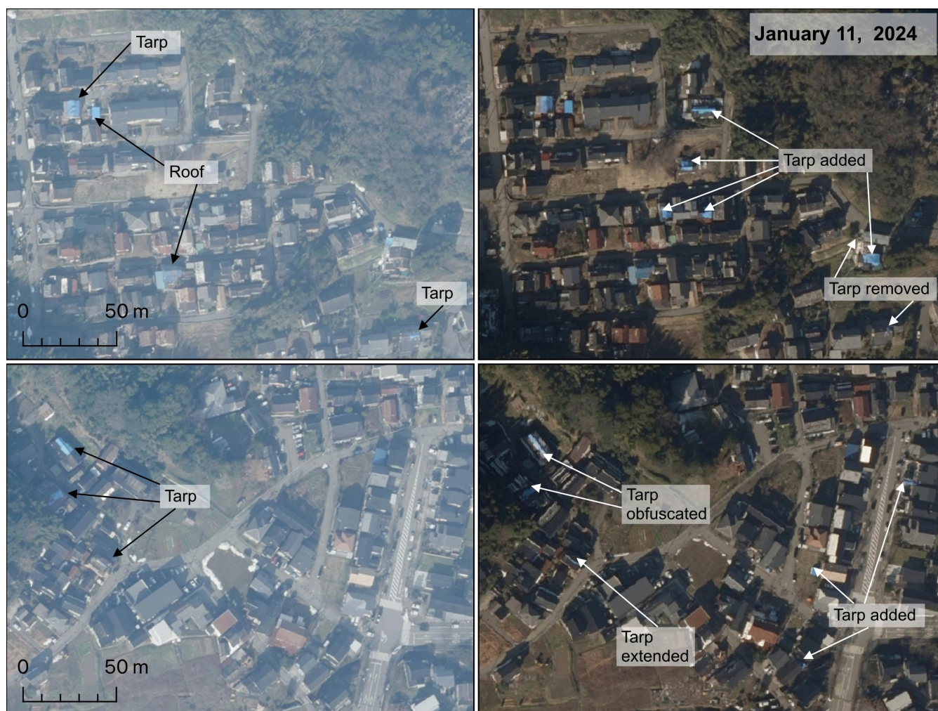
Figure 7. Examples of change in blue tarp coverage in Wajima City between aerial imagery capture missions. The figure highlights challenges faced through potential issues in coverage, atmospheric conditions, and source mismatch. Aerial imagery courtesy of GSI (2024).
