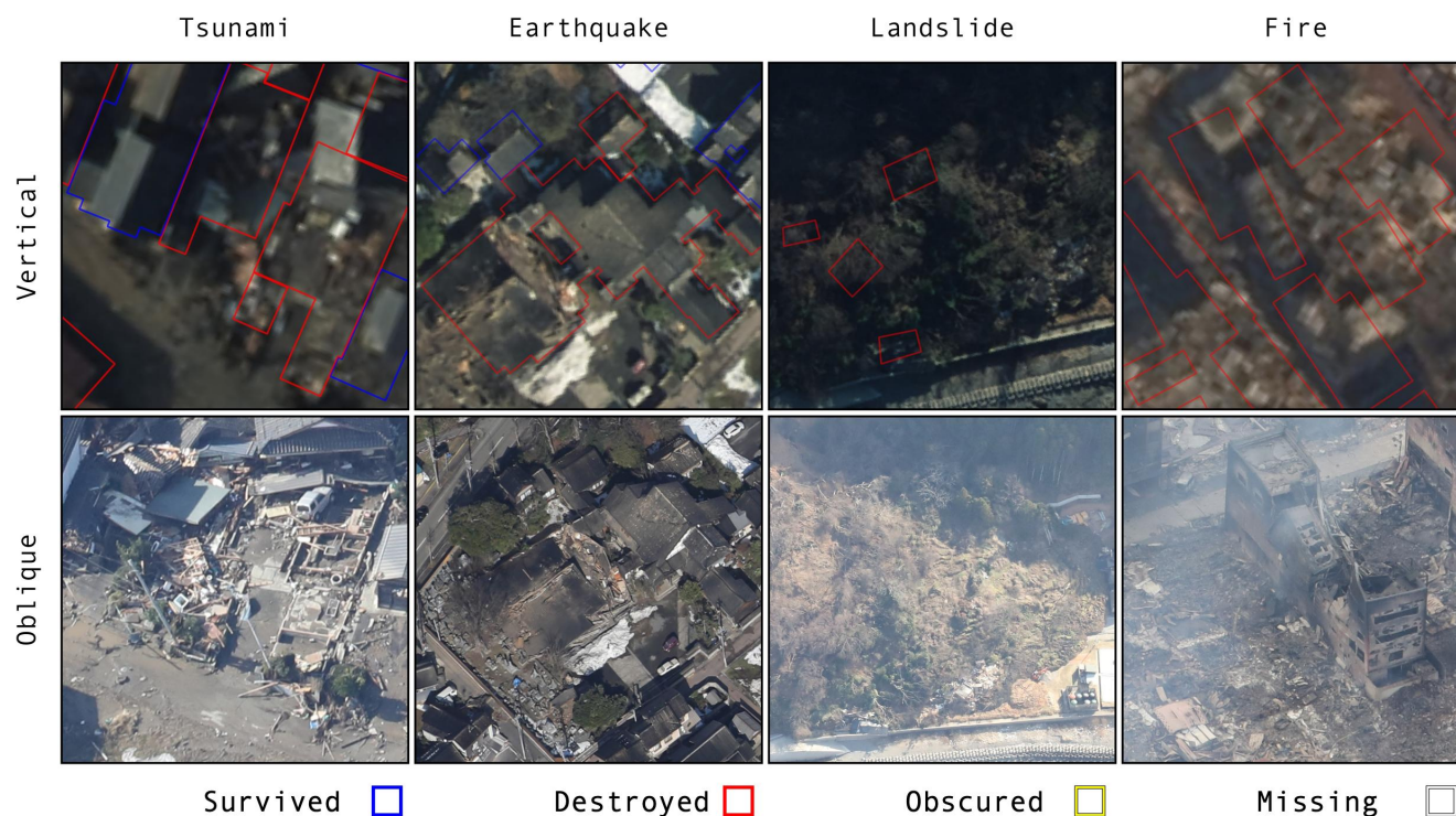
Figure 5. Different modalities of damage consequent to different impacts. Vertical aerial imagery by GSI (2024), Oblique imagery by © KKC (2024)
