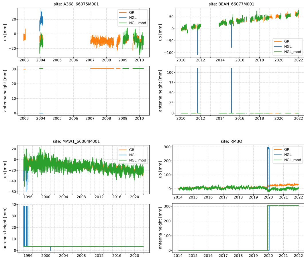
Figure S1. Time series of the vertical coordinate component from the GR (orange), NGL (blue) and NGL_mod with corrected antenna heights according to the GR meta data (green), together with the time series of antenna heights. The sites are selected to demonstrate the effect of false antenna height information on the coordinate trajectory, leading to errors in estimated rates (A368), single outliers (MAW1 and BEAN), or clustered outliers (RMBO).
