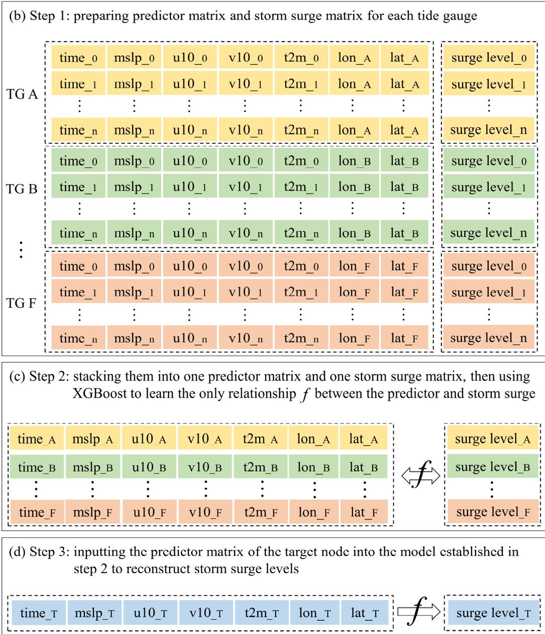
Figure 3: The modeling processes of the ASM framework
