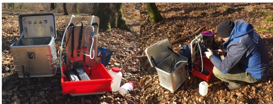
Figure 3. The schematic at the top illustrates the flow-through cell used to measure in-situ electrical conductivity (EC), dissolved oxygen (DO), oxidation-reduction potential (ORP), and pH. The ORP and pH probes were placed in parallel to avoid interference. Two WTW® Multi 3630 IDS data loggers were used to automatically record the probe data. The two photos at the bottom left and right show the setup used in the Weierbach Experimental Catchment and its field application.
