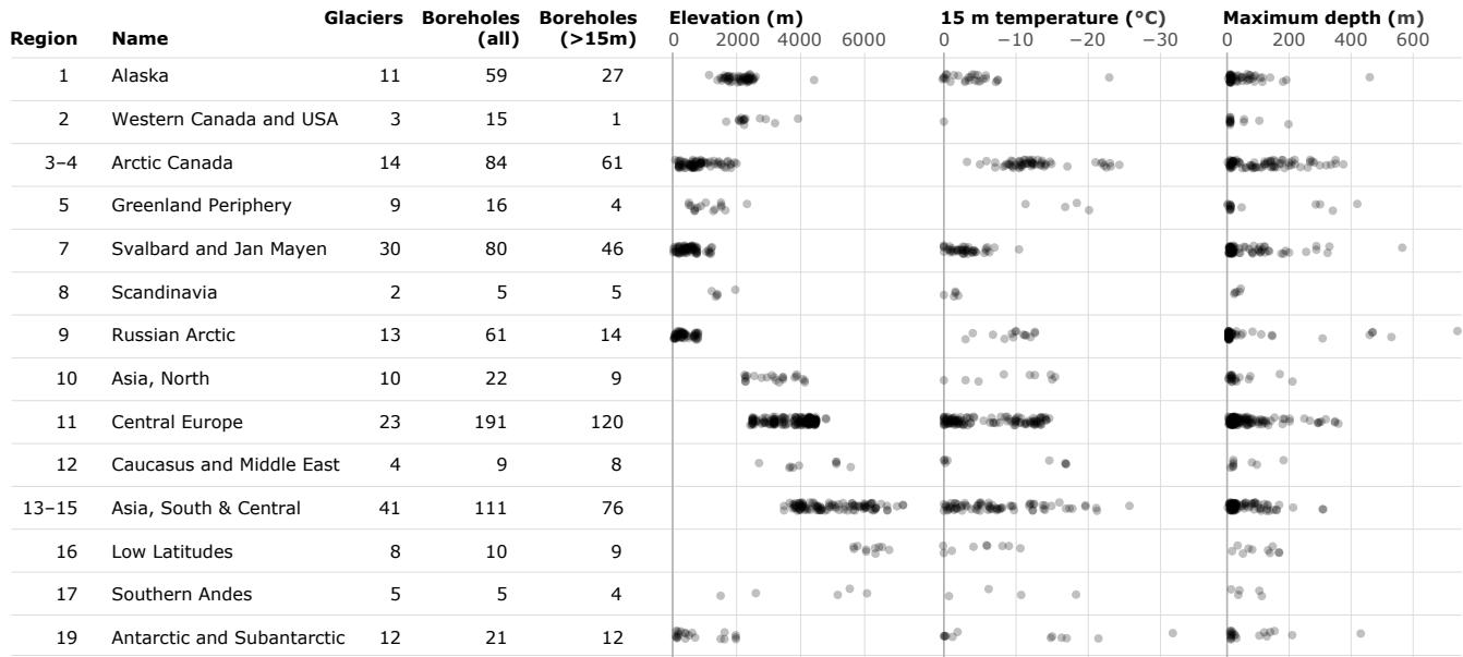
Figure 5. Overview of borehole counts (all and those deeper than 15 m) and surface elevation, 15 m temperature, and maximum measured depth for each borehole (each represented by a dot) by RGI region (see Fig. 3).
