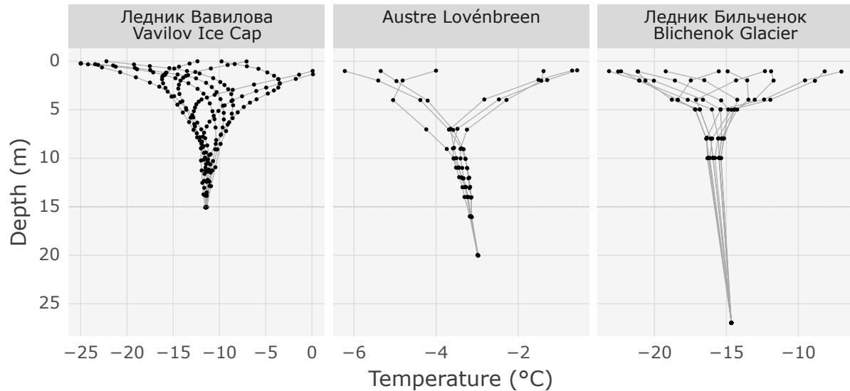
Figure 7. Examples of temperature profiles measured in the same borehole at different times of year, showing the elimination of seasonal surface temperature variations at a depth of around 15 m. Data from Vavilov Ice Cap (Н. И. Барков [N. I. Barkov] et al., 1988), Austre Lovénbreen (孙维君 [Sun Weijun] et al., 2016), Blichenok Glacier (Shiraiwa et al., 2001).
