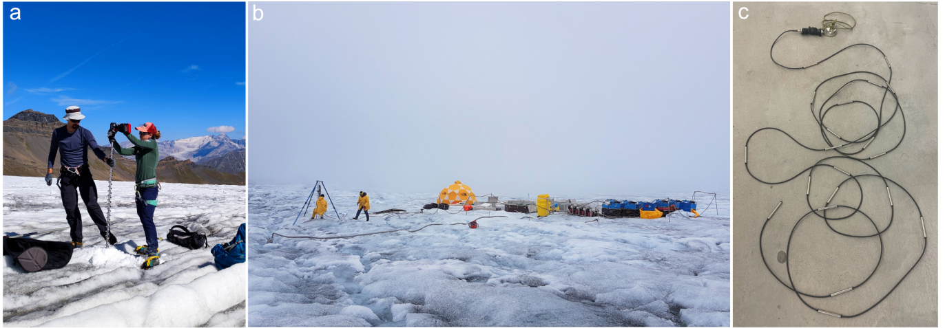
Figure 1. Photographs illustrating methods for measuring glacier temperatures: (a) drilling a shallow borehole with a handheld mechanical auger on Griesgletscher, Switzerland (photo by Matthias Huss), (b) drilling a deep borehole with a hot water drill and a large array of fuel drums and pumps to heat and pressurize the water on Rhonegletscher, Switzerland (photo by Raphael Moser), and (c) a typical string of thermistors used to measure temperature at different depths in a borehole (photo by Mylène Jacquemart)
