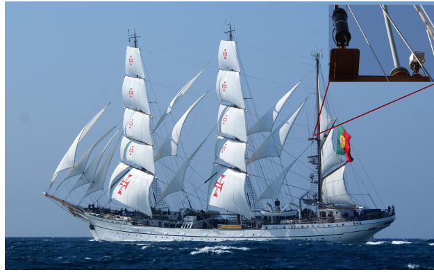
Figure 1. Photo of the NRP Sagres ship in full sail; the inset shows the location on the mast of the gamma radiation sensor (black cylinder, left) and of the primary electric field CS-110 sensor (right).
