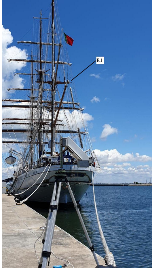
Figure 7. Photo showing the instruments used for the simultaneous measurements of the atmospheric electric field at the mast and on shore.
