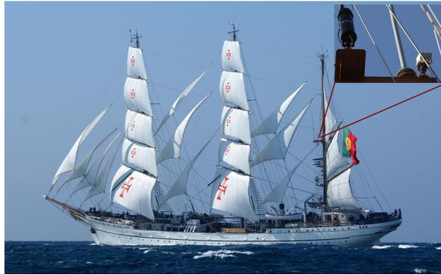
**Figure 1.** [Photo of the NRP Sagres ship in full sail; the inset shows the location on the mast of the gamma radiation sensor \(black cylinder, left\) and of the primary electric field CS-110 sensor \(right\).](#)
