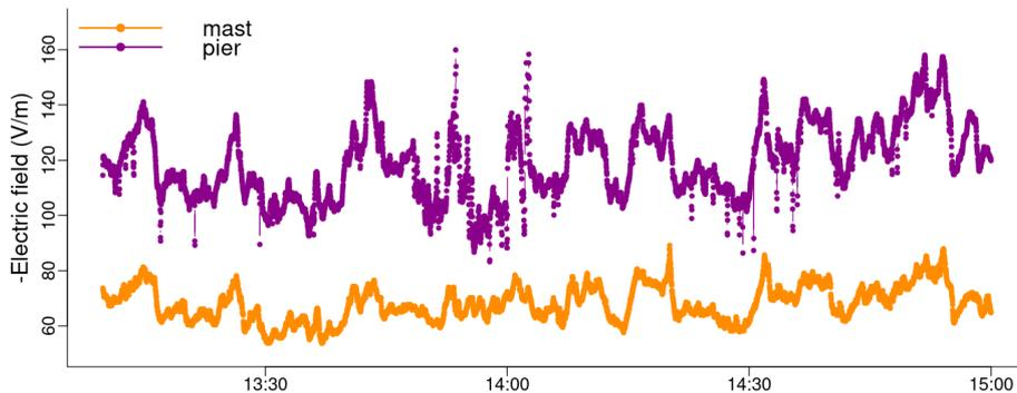
**Figure 8.** Time series of simultaneous atmospheric electric field measurements every 1-second performed at the mast of the ship (at a height of about 20 meters) and at the pier [in Lisbon Naval Base](#) (at the standard height of 2 meters) [under fair weather conditions in 2020-06-16](#).
