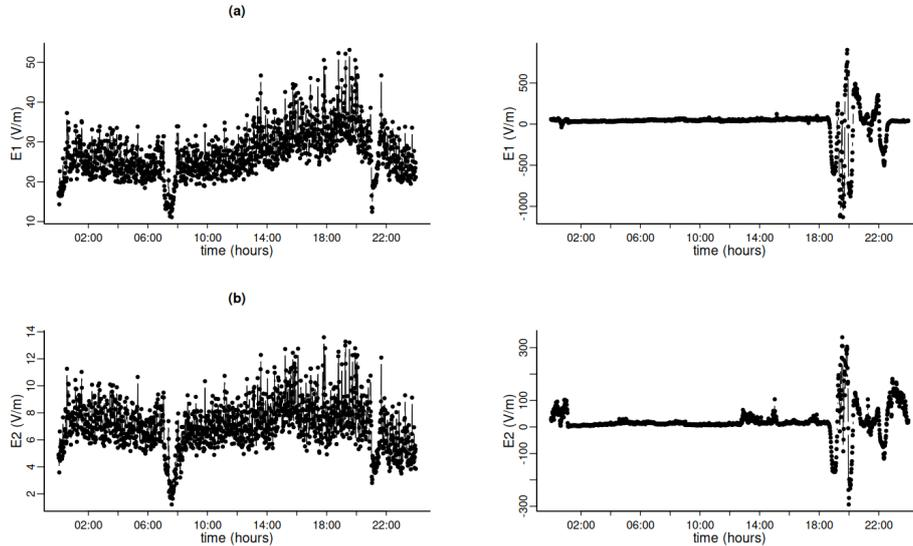
**Figure 6.** Examples of pre-processed electric field observations for a clear day (on February 2nd, left) and for a rainy day (on January 28th, right), from the primary (higher) instrument (top) and the secondary (lower) instrument (bottom).
