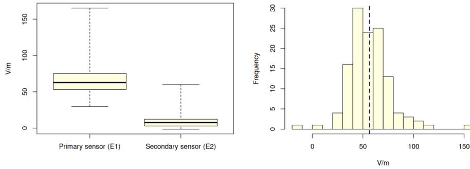
**Figure 10.** Daily median values of height-corrected primary electric field observations and secondary electric field measurements (left) and corresponding daily median differences  $E1_{h\_corr} - E2$  (right), the dashed vertical line representing the average of the differences.
