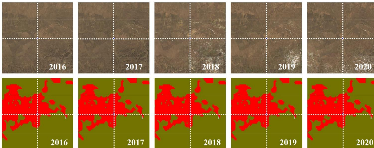
Figure 12. Validation of vegetation mapping: CV sample [100.8570E, 35.2474N] changes detected by CCD not reflected in Landsat and annual vegetation maps.
