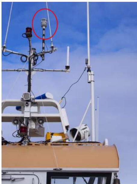
Figure 9. Weather station installed on top of MS Bard/Berg, marked with a red circle.
