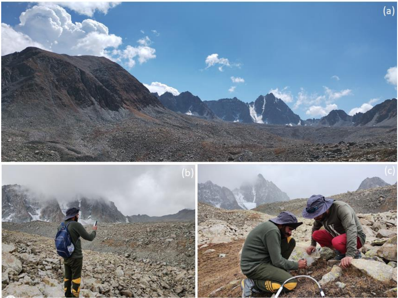
Figure S3. Field photographs of rock glaciers in the Pir Panjal Range: (a) A panoramic view showcasing rock glaciers with RGID (RGU339166N744153E, RGU339244N744189E, RGU339410N744018E, RGU339350N744211E, RGU339293N744283E, RGU339189N744282E), (b) Collecting GPS readings at the toe of the rock glacier, and (c) Installation of ground surface temperature data logger for collecting temperature data in the permafrost landscape
