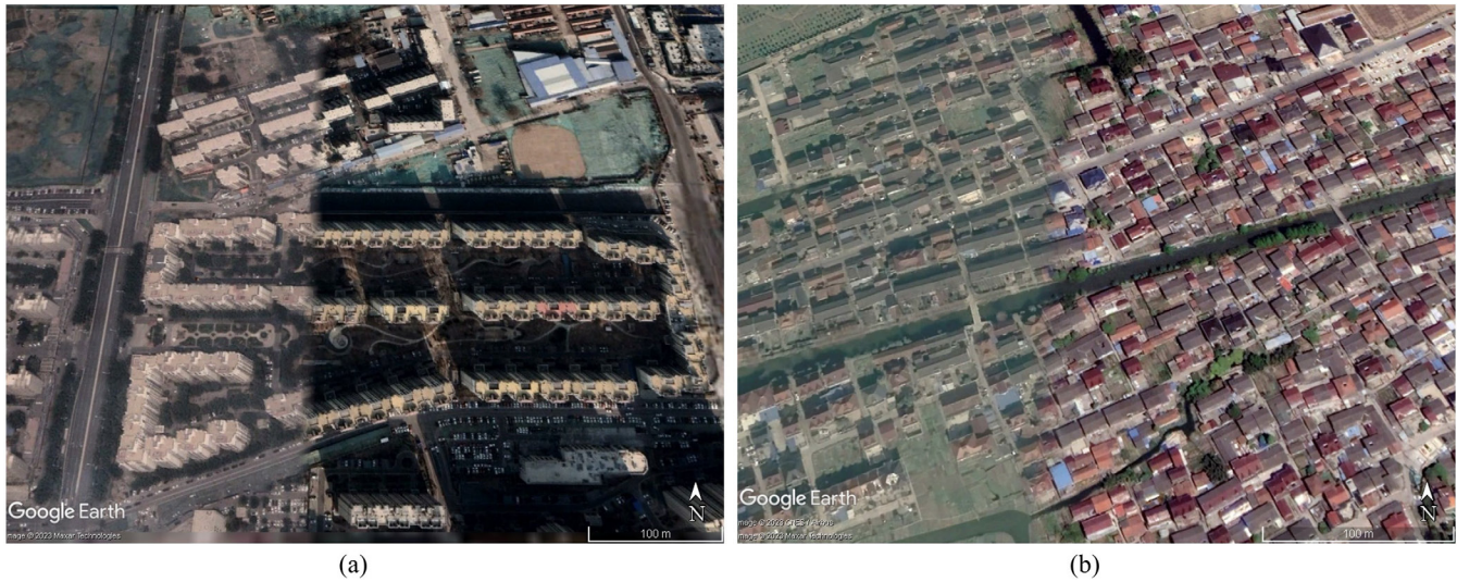
695 Figure A1: Two examples about the stitching part of GES imagery. (a) The high-rise buildings. (b) The low-rise buildings. To acquire larger-scale images, multiple sensors are need to be stitched together, but this process can introduce significant errors at the stitching regions, particularly in areas with height variations like high-rise buildings. The offset is more pronounced in high-rises than in low-rises, as can be seen in the images. Imagery © 2023 Maxar Technologies.
