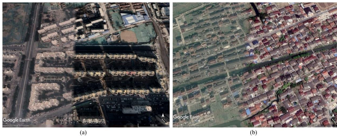
Figure C7: Two examples about the stitching part of GES imagery. (a) The high-rise buildings. (b) The low-rise buildings. It could be seen that the offset is more obvious in the high-rise buildings than that in the low-rises. Imagery © 2023 Maxar Technologies.
