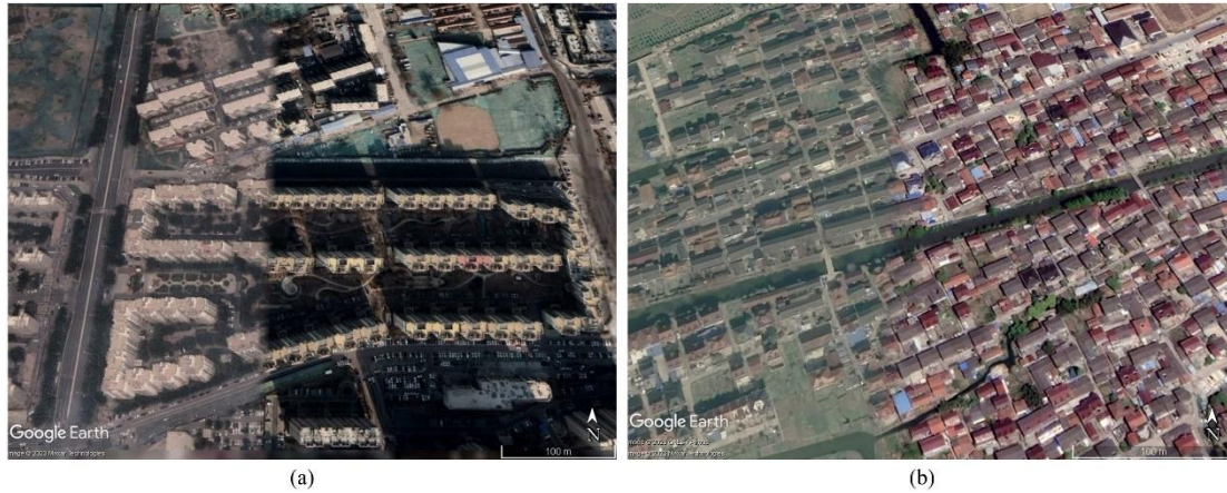
Figure C3: Two examples about the stitching part of GES imagery. (a) The high-rise buildings. (b) The low-rise buildings. It could be seen that the offset is more obvious in the high-rise buildings than that in the low-rises. Imagery © 2023 Maxar Technologies.
