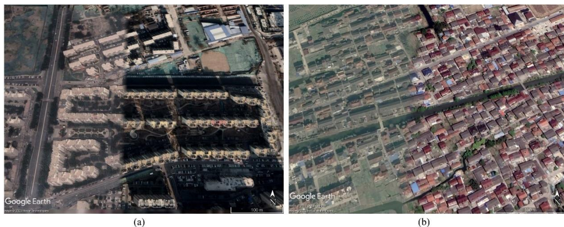
Figure C2: Two examples about the stitching part of GES imagery.(a) The high-rise buildings. (b) The low-rise buildings. It could be seen that the offset is more obvious in the high-rise buildings than that in the low-rises. Imagery © 2023 Maxar Technologies.
