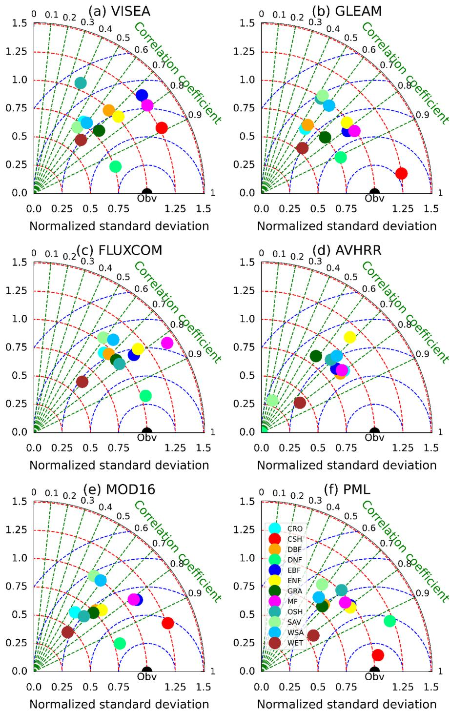
**Figure 7.** Taylor Diagrams comparing monthly measurements of (a) VISEA, GLEAM (b), FLUXCOM (c), AVHRR (d), MOD16 (e), and PML (f) with 150 flux towers (labeled as Obv) in different IGBP land cover types. The diagrams
