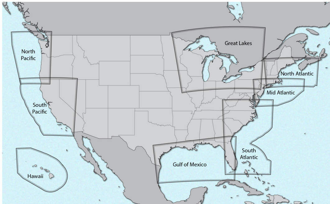
Figure 1. Map of the regional WRF model domains used to build the NOW-23 data sets, masked at the limit of the exclusive economic zone of the countries with jurisdiction on the offshore regions being considered.
