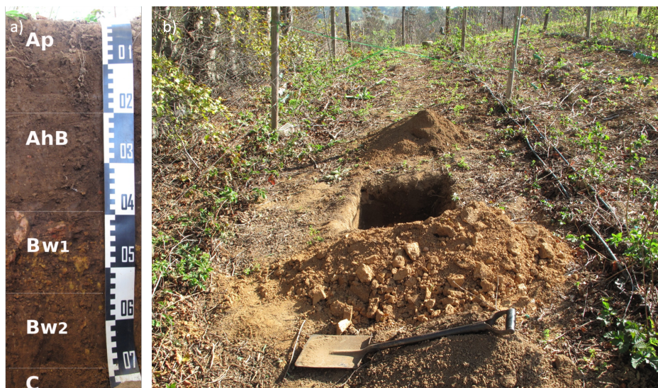
Figure 6. Soil profile: Dystric Cambisol (loamic, colluvic, humic) according to the IUSS Working Group WRB (2015). a) Profile with the delineated horizons, b) profile pit in between the berry rows.
