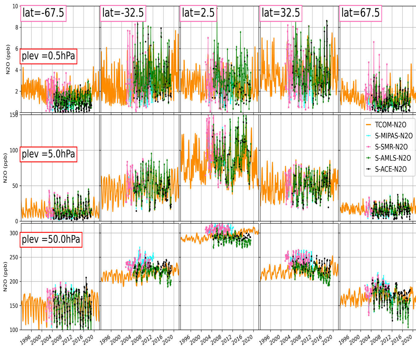
Figure 7. Same as Figure 6 but for \text{N}_2\text{O} . SPARC data from the four satellite instruments ACE (v3.6), Aura-MLS (v4), MIPAS (v422) and SMR (v2.1) are shown with black, green, aqua and pink coloured lines, respectively.
