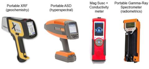
Figure <u>1626</u>: Examples of Core-shed tools that can be used for mineral system characterisation and targeting: a portable X-ray fluorescence analyser (pXRF), portable reflectance spectrometers (ASD), magnetic susceptibility and conductivity meter and gamma-ray spectrometer.
