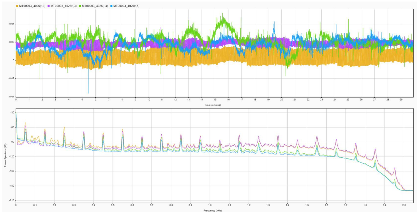
280 Figure 3: Time series (top panel) and power spectra (bottom panel) related to the Electric ( E_x and E_y ) and Magnetic ( H_x and H_y ) field components sampled at 4096 Hz. E_x is plotted in ochre, E_y in purple, H_x in green and H_y in cyan. The components were measured in the (magnetic) N-S and E-W directions. The signal was analyzed in Matlab® Signal Processing Toolbox.
